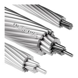
**A** - conductor twisted from aluminum wires. It is used in air atmospheres of types I and II, provided that the sulfur dioxide content in the atmosphere does not exceed  $150~\text{mg/m}^2$  •  $(1.5~\text{mg/m}^3)$  in all macroclimatic regions on land according to GOST 15150-69, UHL execution, except for TV and TS.
